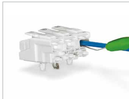
Conductor removal: Slide disconnection tool beneath the conductor and pull conductor out.
